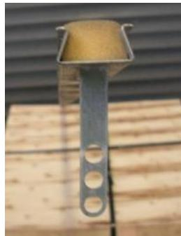
The **Wall connection anchor (AS)** for thin-bed mortar joints is hooked into the built-in wall connection rail MAS 25/15 or into the anchor rail 28/15 and pressed into the mortar of the wall joint until the holes of the wall connection anchor are filled with mortar.
