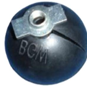
**BGW pocket former (ASK) narrow** is made of rubber and is used to fix capstan lifter in narrow components, on or in the formwork. Either the fixing nut or the fixing screw is installed in the pocket former. The KKA is inserted into the open recess mouth. When fastened to the formwork, the jaw of the pocket former is closed by screwing in or tightening the screw in order to ensure a secure fit of the KKA.
