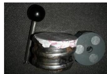
To prevent cement glue from penetrating the opening and damaging the built-in part and the magnet system, the built-in part is sealed with adhesive tape.
