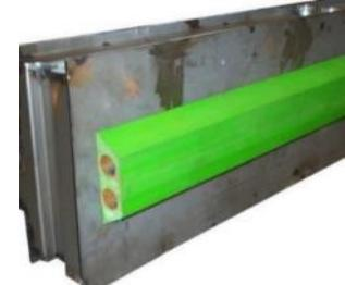
It is essential to ensure that the shuttering systems are not placed on top of each other with the adhesive side. If this is the case, the systems must only be pushed apart laterally (do not pull them apart, otherwise the magnets will be torn out of the plastic)! In case of improper handling, we cannot give any guarantee!
