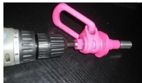
These HFAMs can then also be used as a better alternative such as a transport anchor for double walls. To realize this, these are installed on both sides of the double wall.
