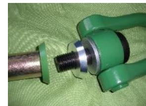
For fixation on steel formwork BGW-Magnets Type HM4-D are recommended. BGW-segment anchor lifter supports itself by its geometry on the flanks of the recess. This relieves the tension on the threaded pin and allows greater transport safety.
