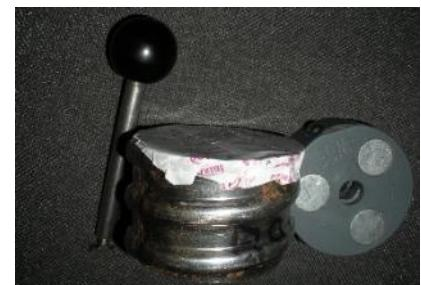
To prevent cement glue from penetrating the opening and damaging the built-in part and the magnet system, the built-in part is sealed with adhesive tape.
