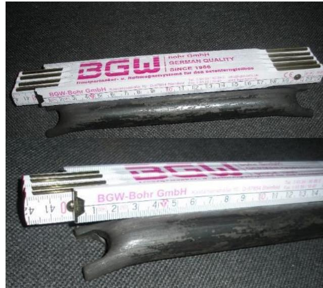
Length of the pipe cross brace for anchor bracket Load level 3.7t = concrete wall thickness - 74mm, for 4.5t - 75mm, for 5.8t - 78mm, for 8.5t - 82mm
