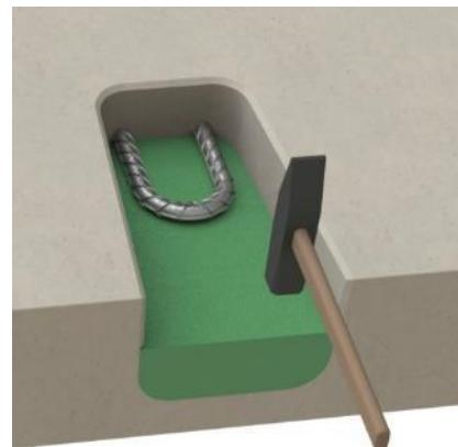
Light hammer blows on the pocket former can facilitate demoulding
