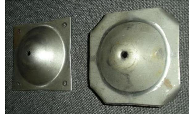
The Ø 8mm centering pin is hammered into this hole, the centering pin is about 50mm above the concrete.
