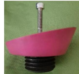
The main feature of this retaining washer is that it is inclined on the side facing the formwork and therefore lies flat against the formwork when the threaded anchor is to be installed in a component "at an angle" - i.e. in the direction of pull, i.e. in the extension of the sling.
